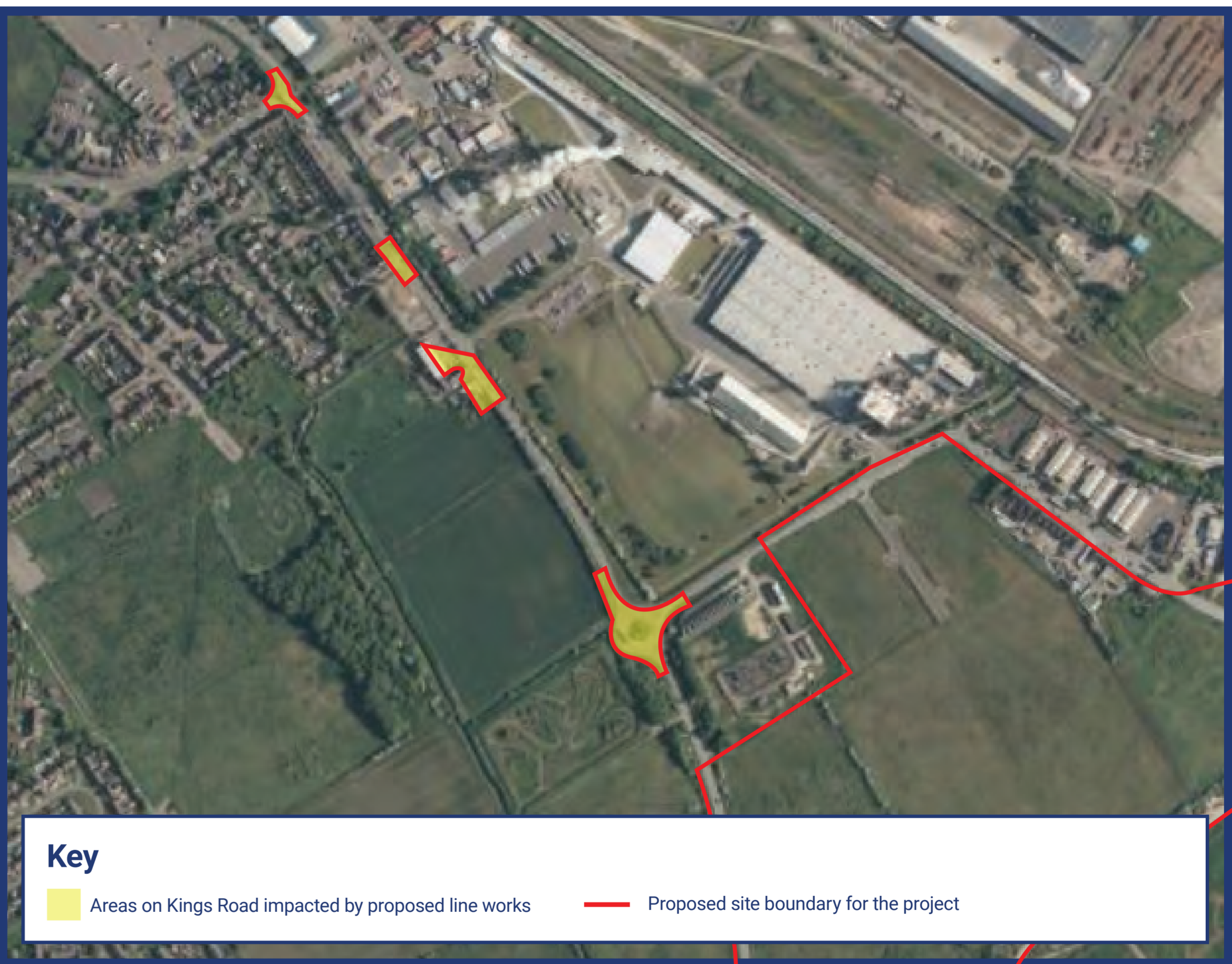
This image shows areas where overhead line works may be needed to facilitate delivery of construction materials
