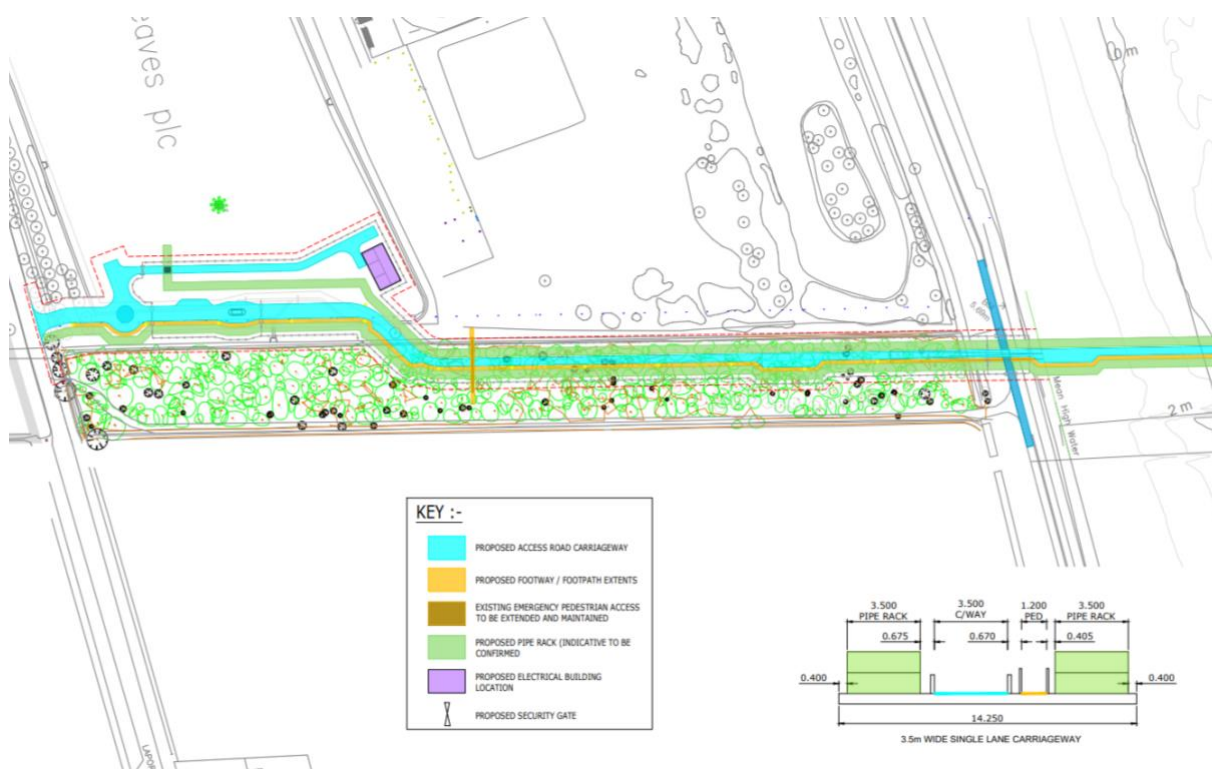
Plate 6.2: Illustrative Pipe Rack and Jetty Access Road design (revised)
